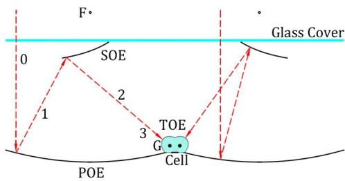
**Fig. 1.** Two-dimensional sketch of the rays' paths for the transverse section of two optical units through a module's diagonal. (0) Incoming sunrays; (1) reflected rays on the primary optics; (2) reflected rays on the secondary optics; (3) rays transmitted through the tertiary optics and impinging the solar cell. The foci of the two-sheeted circular hyperboloid are (F) and (G), where (F) is also the circular paraboloid's focus.
