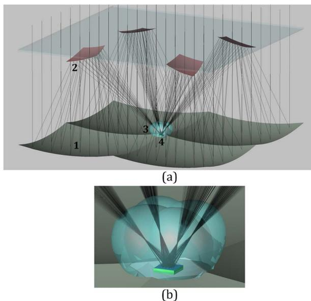
**Fig. 2.** (a) Model and ray tracing of the Cassegrain 4-optical-unit module with the central receiver. The elements are marked: (1) paraboloid mirrors (POE), (2) hyperboloid mirrors (SOE), (3) homogenizer (TOE), and (4) solar cell. (b) Detail of ray tracing at the central receiver.
