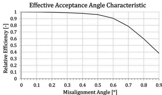
Fig. 4. Effective acceptance angle characteristics of the design.
