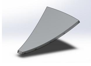
Fig.4 Trapezoidal reflective petal of solar parabolic concentrator
