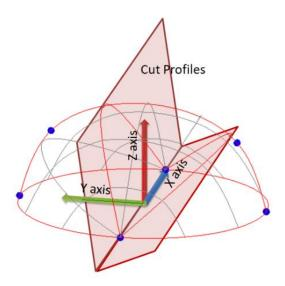
Figure 2. Freeform slice surface made using cut profiles.
