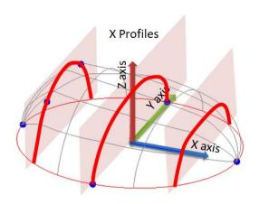
Figure 1. Freeform slice surface made using x profiles.
