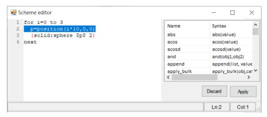
Figure 7. Once in step execution mode, use the F11 key to step through execution line by line.
