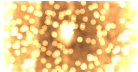
Medium Setting – 30 Minutes, Moldtech Texture on output face, much better uniformity
