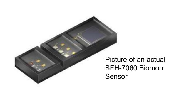
LED supplier OSRAM has its own all-in-one sensor featuring three LEDs emitting at 940 (infrared), 655 (red), and 530 (3x green) nanometers and a photodiode in an extremely small package, 4.7mm x 2.5mm by .9 mm with a light barrier to block optical crosstalk. This OSRAM biosensor is a good off-the-shelf component to monitor pulse rate and provide pulse oximetry information for a wearable.
