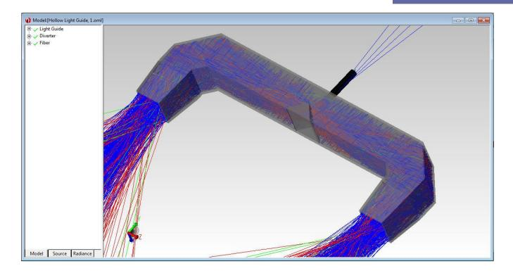
Not all light guides use TIR. An example is a hollow light guide with a reflective interior for a UV application.
