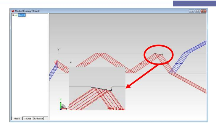
Add a physical feature to the surface of the light guide. An example would be a backlight light extractor.
